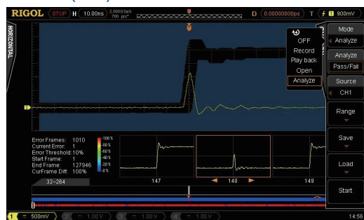
Real-time waveform recording, playing, and analysis function (Std.)
